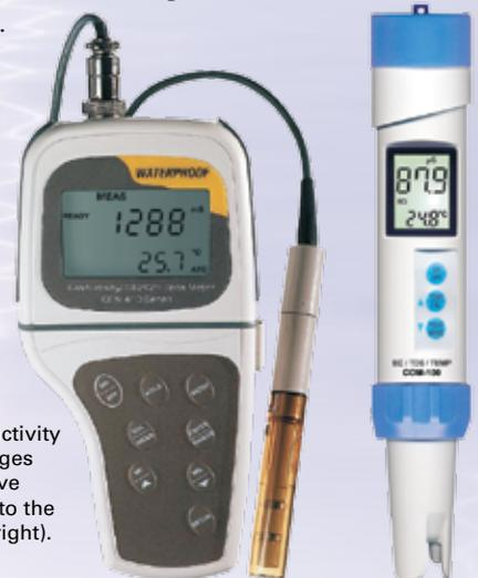
**Figure 1:** Popular styles of conductivity meters: Availability ranges from the more expensive laboratory grade (left), to the cheaper, pocket-sized (right).
