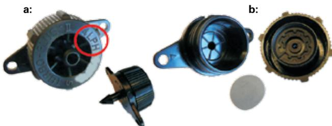
**Figure 2a:** This pressure compensating dripper delivers exactly one gallon per hour provided the delivery pressure is 100-400kPa.
