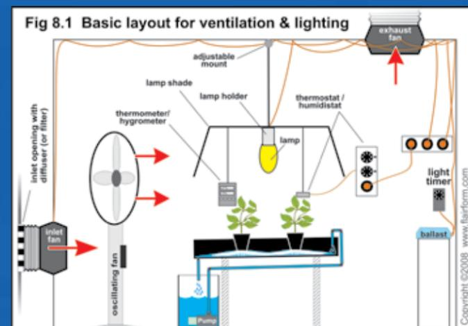
Figure 1. Basic layout for ventilation and lighting.
