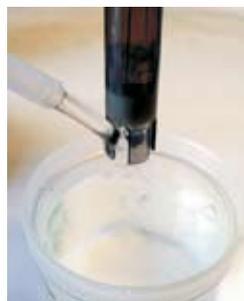
**Figure 4:** Always clean the electrode with distilled water after use - No. 1 maintenance tip for prolonged electrode life!
