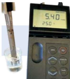
**Figure 2:** Stir nutrient tank well before sampling. Then leave the electrode in the sample for a few minutes before switching the meter on and taking the measurement.
