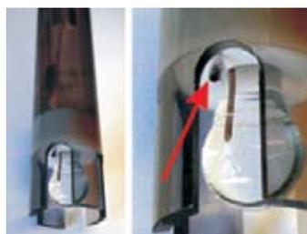
**Figure 7:** Arrow highlights contamination on this 'frit' (or wick). The hydrogen ion sensitive glass 'bulb' containing the measuring cell electrode can be seen to the right of the arrow.
