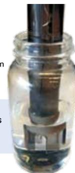
**Figure 5:** Always keep pH electrodes immersed in a "storage" solution when not in use.
