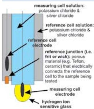
**Figure 6:** Schematic layout of glass pH electrode. Loss of accuracy is invariably explained by different degrees of blockage of the 'frit' or 'wick' - often caused by dry storage. Testing of oily or harsh chemicals (eg. pH Up or concentrated nutrient), or failure to rinse the electrode properly after use.
