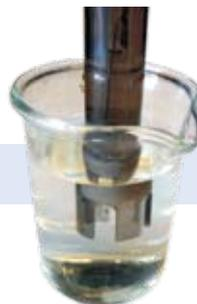
**Figure 3:** Do not immerse the electrode deeper than 20mm.
